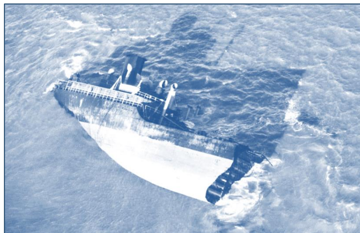
Figure 2-1: The catastrophic Liberty Ship tanker failures during cold weather were a landmark case that led to further development of fracture mechanics.
