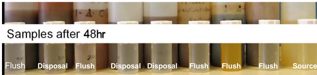
Figure 15 – Water samples before and after settling for 48 hours for T10.
