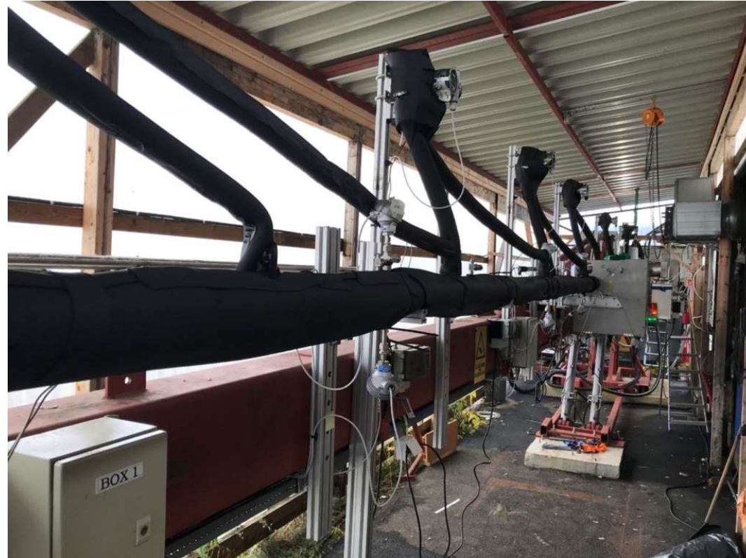
Flow Assurance Loop for CO 2 transport
