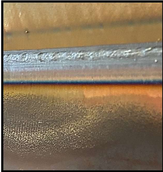
As-welded root profile
