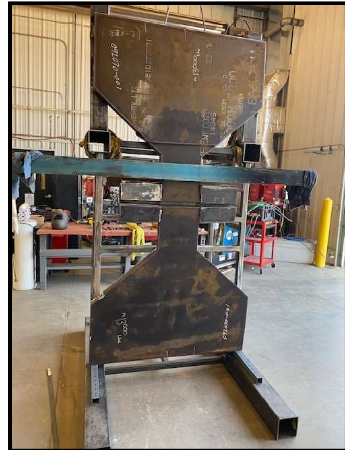
8' x 4' Fatigue Specimen 2.76 inches thick
