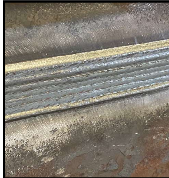
As-welded cap profile
