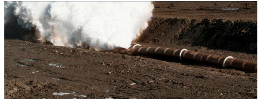
CO2 Fracture Propagation Test – EPCRC 2017
