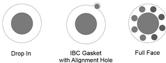
Figure 6.4.3.1b - Types of gaskets
