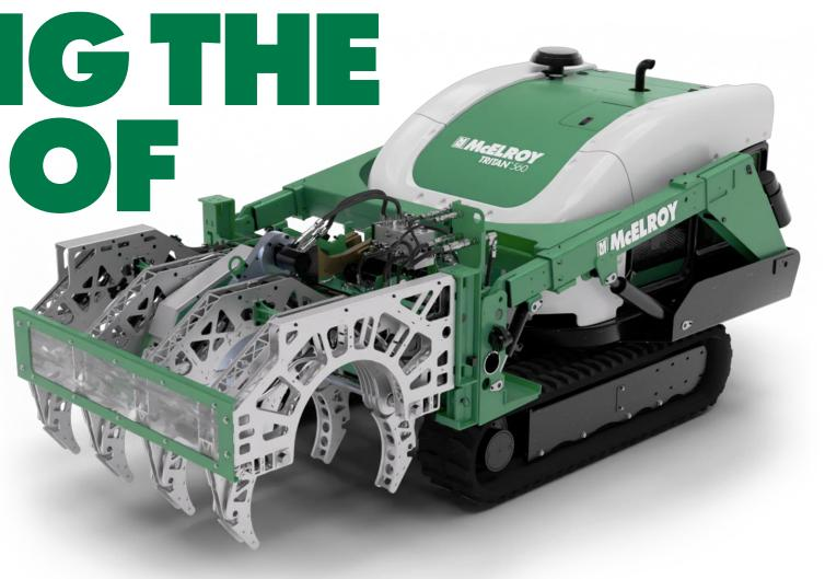
Vehicle with 360-degree rotating frame allows machine operators to fuse in front of, or parallel, to the tracks on either side of the machine.
