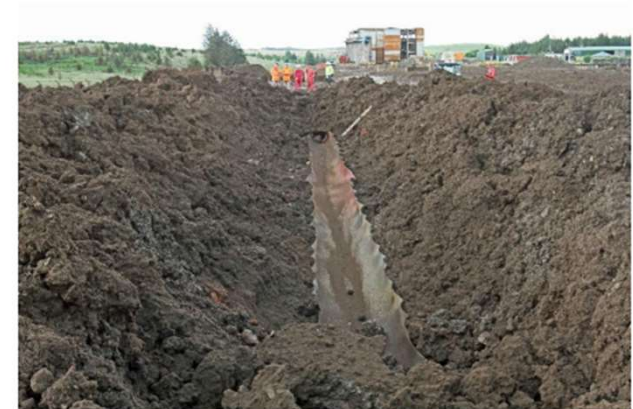
Running Ductile Fracture in Dense CO2 Pipeline – Experimental Test [9]
