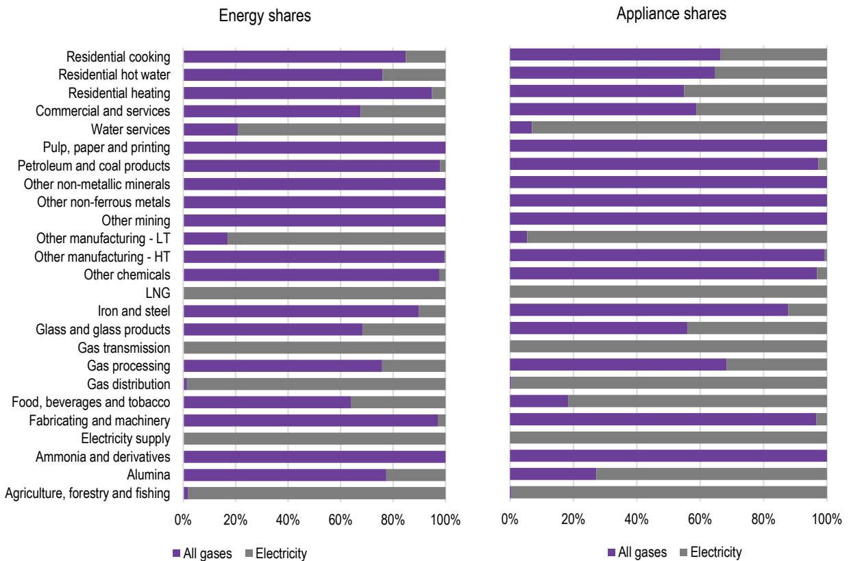
Figure 3.41 Energy and appliance shares by sector and fuel type in 2050: Accelerated RGT scenario
